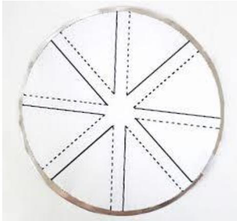
2. Taking each blade, bend one side gently up (along the dashed lines) so that all blades are curved up the same direction.
